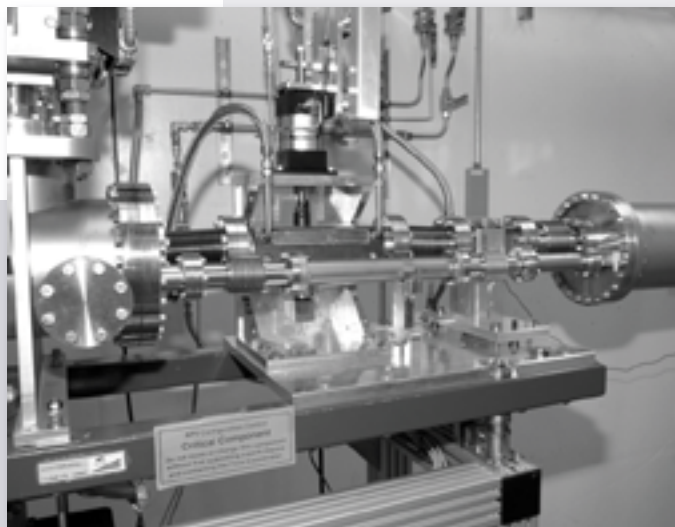
Split Beam – The two separate beamlines exit the cylinder at the right. They begin just hair-widths apart and spread to two feet apart over the 60 meters they travel together.
