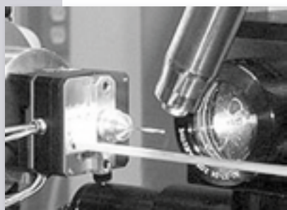
Sample Area – This close-up of the area where the sample is placed shows the on-axis visualization lens that designers incorporated to make the beamline easier to use.
