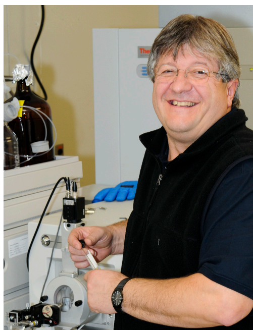
Josip Blonder, M.D., Laboratory of Proteomics and Analytical Technologies, prepares to insert a new ion transfer line into the mass spectrometer (MS) source for a hybrid (ion-trap/FTICR) state-of-the-art MS instrument.
