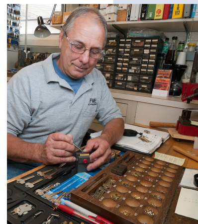
Tim Gibbs sets a lock in the FME shops before installation.
