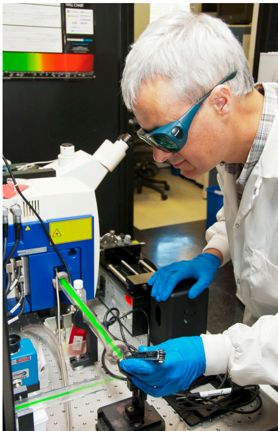
Stephen Lockett aligns the beam of a two-photon microscope so that the sample is efficiently and evenly illuminated. For deep imaging into tissue samples, usually living samples, it is necessary to excite the fluorescence-tagged proteins in the sample with two photons instead of one. The laser light (shown in the tube) is simulated in the picture. Photo illustration.
