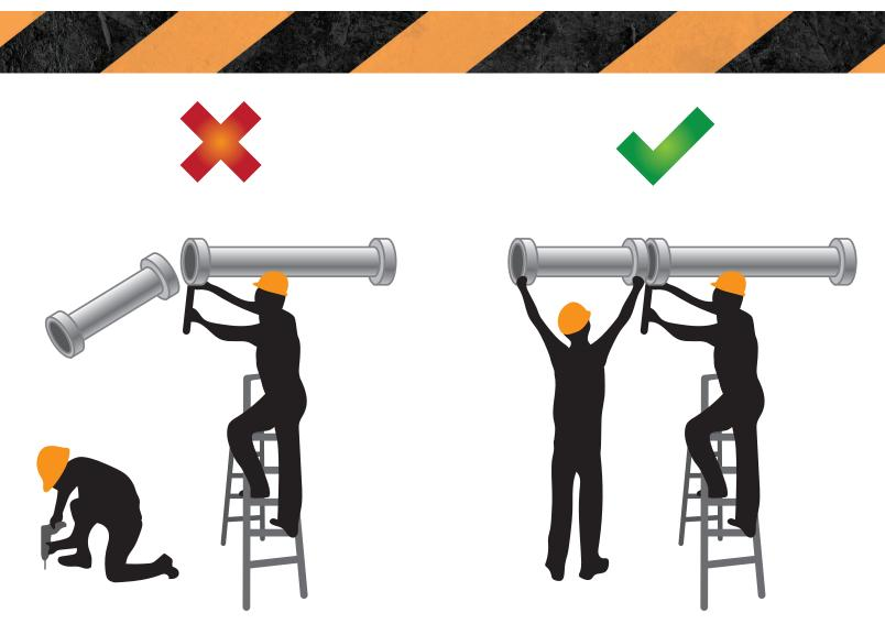
**OVERHEAD/DROP HAZARDS** exist in demolition and construction Workers can be **STRUCK BY**, **CRUSHED**, or even **KILLED** by overhead loads
