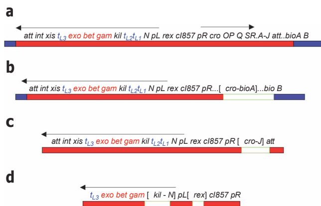
Figure 7 | Schematic representation of \lambda phage constructs used for recombinering. (a) The \lambda prophage with some of its genes is shown integrated in the bacterial chromosome. It is adjacent to the biotin gene bioAB . Bacterial DNA is shown as a blue bar; phage DNA is shown as a red bar, and a region containing a deletion and/or a substitution is shown as a white bar in b–d. The complete \lambda prophage is flanked by its attachment sites att , where integration occurred. The int and xis genes located in the pL operon encode functions to integrate and excise the phage DNA into and out of the bacterial chromosome. Two operons with their promoters pL and pR are indicated. Transcription of the promoters is controlled by the \lambda CI857 repressor. This repressor is temperature sensitive in that it is active and represses the promoter at 30–32 °C but is inactive at 42 °C allowing for transcription. The N protein functions as a transcription anti-terminator and prevents RNA polymerase termination of pL transcripts at terminators tL1 , tL2 and tL3 . The red genes exo , bet and gam encoding the homologous recombination functions are also in the pL operon. The kil gene is adjacent to gam and, when expressed for over 1 h, kills the bacterial cell 32 . The replication genes O and P are in the pR operon. Cro functions as a partial repressor of the pL and pR operons when CI is inactive at 42 °C. The lysis and structural genes, SRA–J , are shown located beyond their regulator Q . The \lambda TetR phage used for recombinering is identical to the above complete prophage with the exception of four changes. The replication gene P has an amber mutation, the cro gene also has an amber mutation, and the tetA gene encoding tetracycline resistance replaces rex . (b) The defective prophages in DY380, SW102 and the HME strains have the lytic pR operon deleted from cro through the bioA genes as shown in brackets. The right att site is also deleted, preventing any excision of this prophage. In DY380 and SW102, cro through bioA is replaced by the tetracycline resistance cassette, tetRA . (c) The mini- \lambda phage DNA is shown with the lytic genes cro through J deleted. In different constructs of the mini \lambda , the cro–J region is replaced with various drug-resistant cassettes. Mini- \lambda has both att sites plus int and xis , which allows for its integration and excision. (d) The \lambda segment on the pSIM plasmids is shown. The plasmid backbone is not shown. The genes from cro to att are removed as well as genes beyond tL3 , including int and xis . The red genes are connected directly to pL by a deletion that removes kil through N . The drug-resistant marker characteristic of each SIM plasmid replaces the rex gene adjacent to CI857 . The basic features are conserved in all of these Red expression constructs. Red is left under the native phage-controlling elements for optimal expression and regulation. The pL promoter drives gene expression and is controlled by the temperature-sensitive but renaturable \lambda CI857 repressor. In all, the cro gene is inactive to maximize pL expression, and the replication genes are absent or inactive to prevent lethal effects on the cell.
